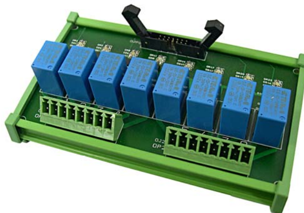
Figure 4 Output module - Relay
